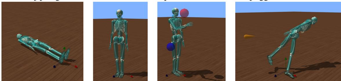
Figure 1: From left to right, behaviors of the cumulative control modules for posing, standing, and reaching. The last one shows the standing controller reacting to external perturbations.
